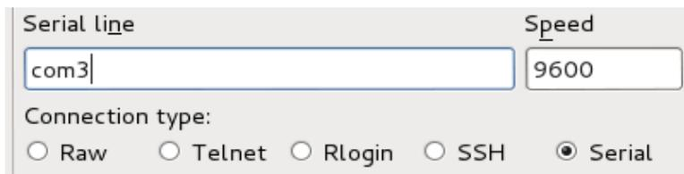
The image shows the PuTTY configuration dialog box. The 'Serial line' field contains 'com3' and the 'Speed' field contains '9600'. Under 'Connection type', the 'Serial' radio button is selected, while 'Raw', 'Telnet', and 'RLogin' are unselected, and 'SSH' is also unselected.
